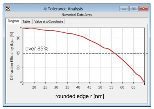
Rigorous simulation with Integral Method (IM), for tolerance analysis over 30 steps, takes 9 seconds.
