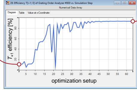
parametric optimization – downhill simplex method – with rigorous Fourier modal method (FMM) used for grating efficiency calculation
