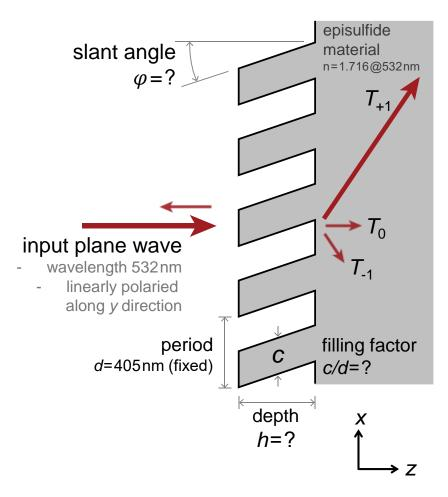
How to optimize the  $T_{+1}$  order diffraction efficiency, by adjusting the slant angle  $\varphi$ , grating depth h, and filling factor c/d?
