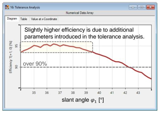
Rigorous simulation with Fourier modal method (FMM), for tolerance analysis over 50 steps, takes 30 seconds.
