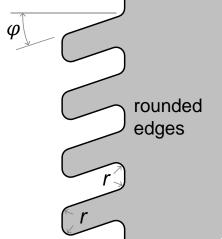
In addition, how to evaluate the grating performance with the slope deviation and the rounded edges due to the fabrication technique taken into account?
